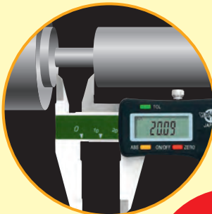
Measurement on edge face (measurement with flat-head)
