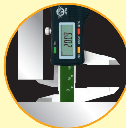
Measurement of height from a face
